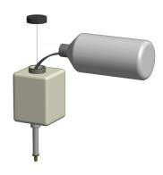
7. Mount the pump housing by gently sliding it back into the slot
