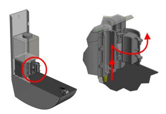
3. Remove the soap container by gently pulling it out of the pump housing.
