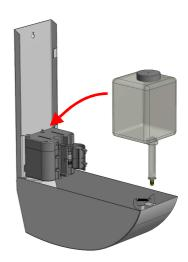
Pull silicone tube downwards and place the outlet nozzle in the slot. Make sure that the collar is located under the pump housing.
