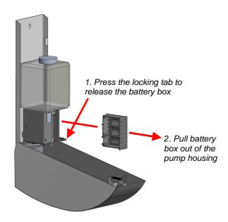
3. Replace the three C type batteries. Be aware that they must be properly oriented with polarity as shown on the illustration.
