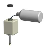
Mount the soap container by gently pushing it into the groove on the pump housing.
