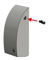
2. Open the flap on the front of the pump housing by gently lifting it approximately 1 cm and turn it anti clockwise.
