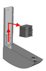
Mark the holes on the wall at the chosen location by using the enclosed drilling template.
