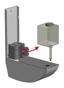
Remove the cap and fill the soap container with appropriate liquid soap.
