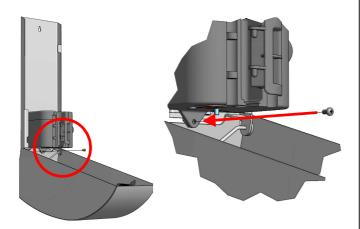
11. Pull silicone tube downwards and place the outlet nozzle in the slot. Make sure that the collar is located under the pump housing.
